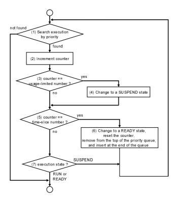
Fig. 5. Process flow when the directory execution with an upper bound is found
