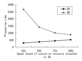
Fig. 8. Processing time when the upper bound of the execution resource attached to SB is changed
