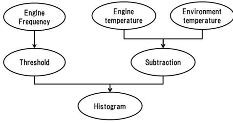
Fig. 3. An example of flow in aggregation processor
